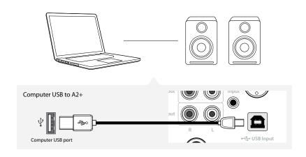
For PC, the A2+ should be recognized automatically.
